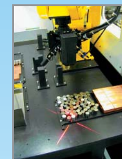
Automatic workpiece search by 3D sensor
