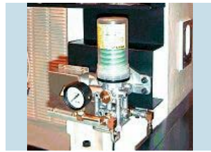
Auto grease lubrication system
